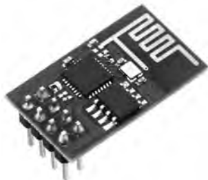
Fig. 6. ESP8266 microcontroller board
