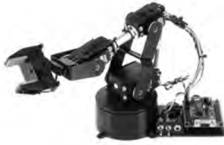
Fig. 10. AL5A robotic arm with SSC-32 controller board [25]
